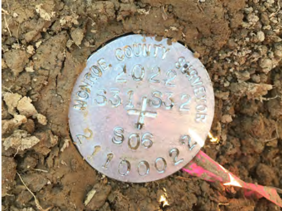
Photo Orientation & Description: Capped rebar at E25
