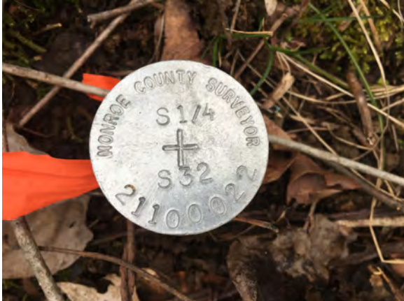
Photo Orientation & Description: Capped rebar at G25
