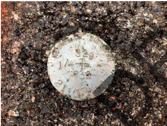
Photo Orientation & Description: Capped rebar at G21
