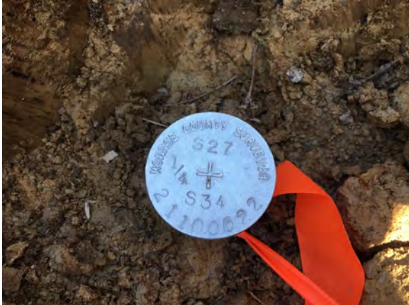
Photo Orientation & Description: Capped rebar at O21
