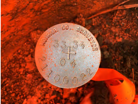
Photo Orientation & Description: Capped rebar at M25
