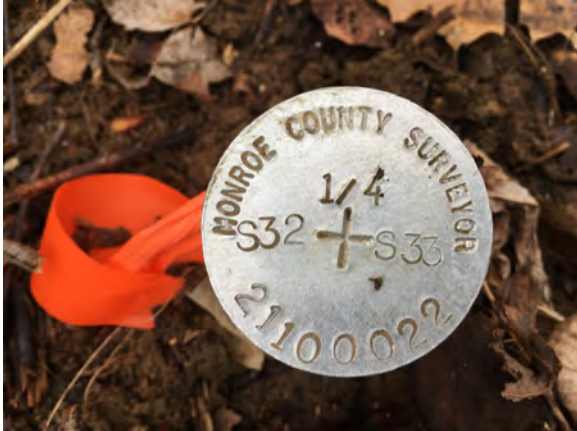
Photo Orientation & Description: Capped rebar at I23
