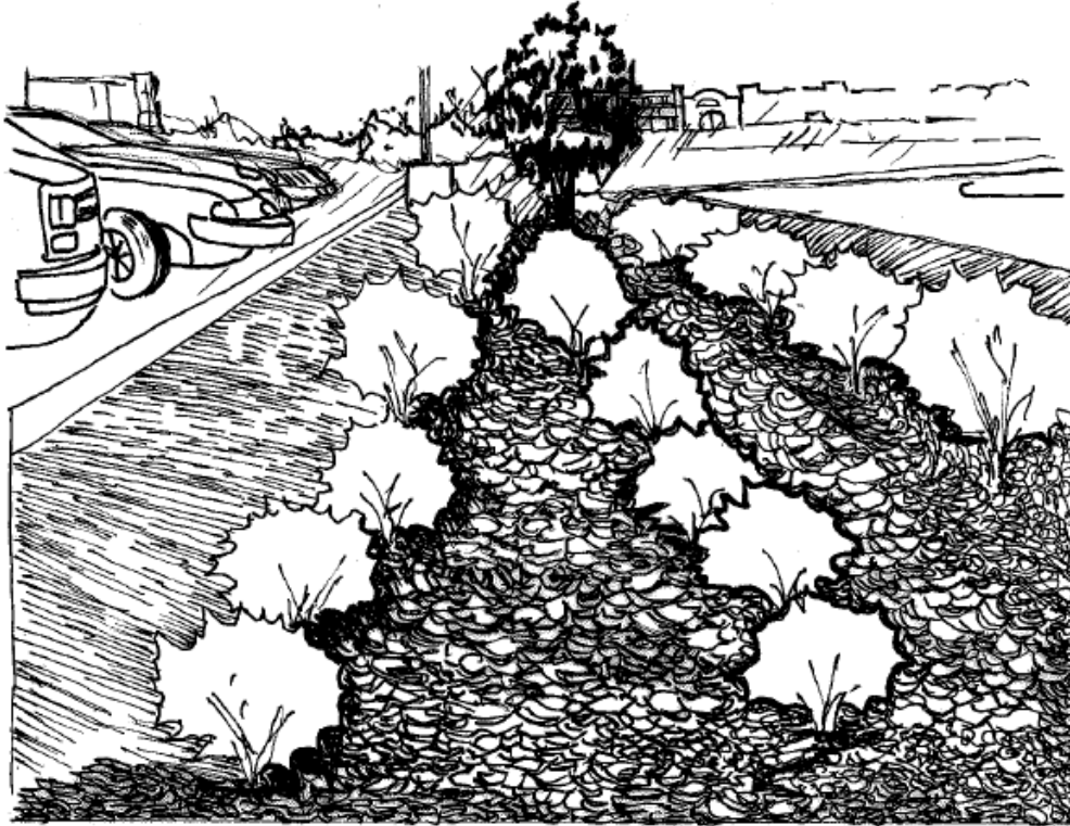
Figure 30-9 Parking Lot Landscaped Strip Bioretention for parking lot perimeter or between rows of parking spaces.
