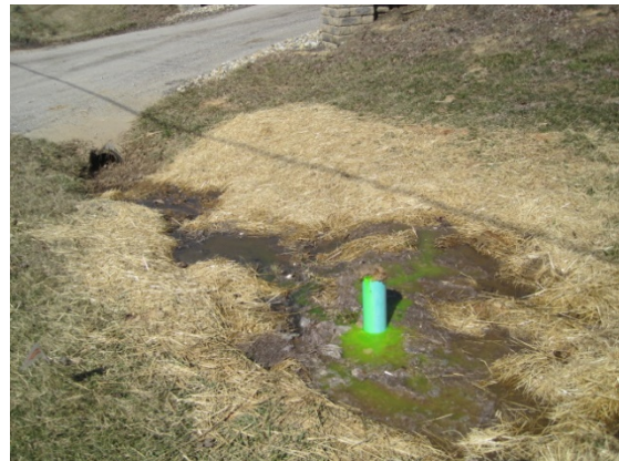
Colored tracing dye confirms a raw sewage discharge in Monroe County
