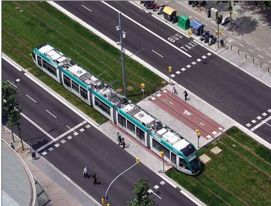
Figure 6: Light Rail track in a median. Source: railway-technology.com
