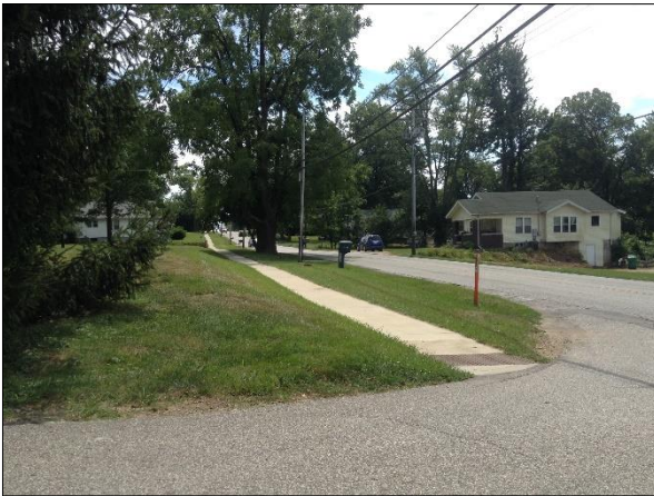
A rural/suburban collector sidewalk is a hard surface path along a major street with no curb and gutter.
