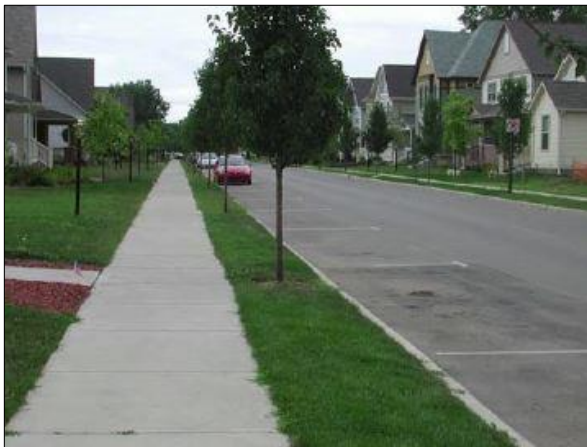
An urban residential sidewalk is a hard surface path along a street with curb and gutter, ideally separated from traffic with a buffer strip or corner curb extensions.
