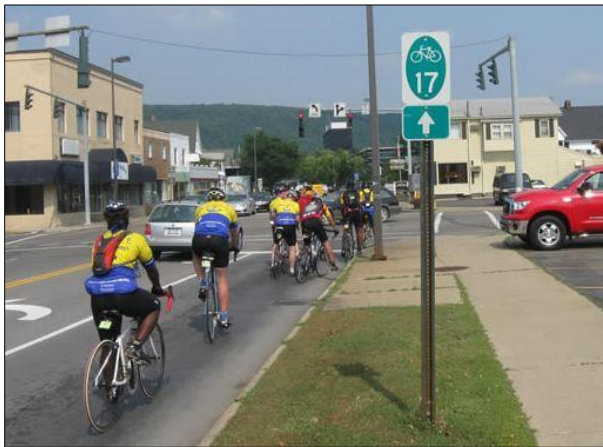
A signed bike route is a street that is safe for use by both vehicles and bicycles without a designated bicycle facility, but with appropriate signage.
