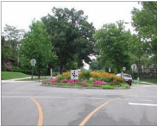
Traffic circles, or roundabouts, can be traffic calming when designed effectively.
