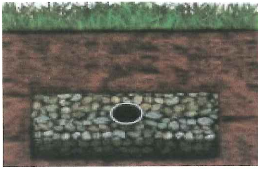
Septic field comprised of river rock
