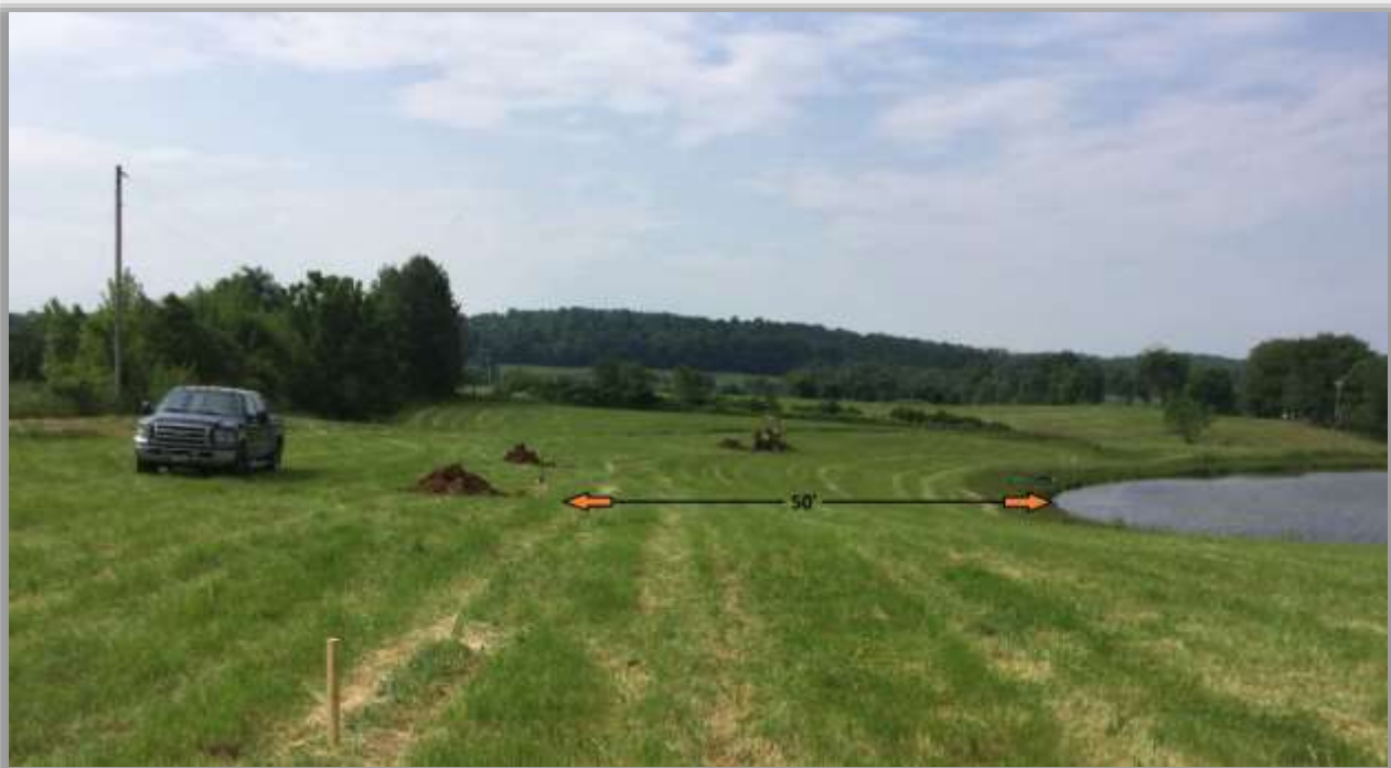
This picture shows the on-site investigation of a property for a septic leach field by the soil scientist using backhoe pits to determine soil properties. In addition, on all new construction, the soil scientist observes on-site features such as bodies of water (ponds, lakes or streams). Here, the required 50 feet set-back from the pond is identified prior to conducting the soil investigation with the backhoe pits.
