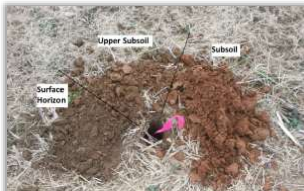
During the on-site investigation our staff soil scientist commonly uses a 4 inch diameter boring auger to examine the soil properties to a depth of 60". The soil report will identify specific soil horizons and the observed properties at each horizon depth. At this boring location the soil has been placed to show the progression from surface 0 to 60" depth. Notice the bright browns and red colors that indicate a well-drained soil profile.
